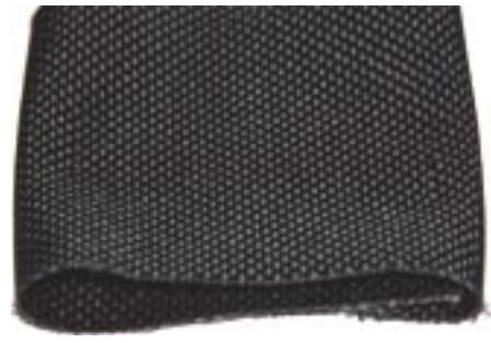
Ballistic Nylon (BN) 1/16" Thick
