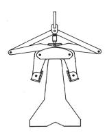
4. Slack in hoist line will engage auto-latch, holding grab open for removal and placement of next barrier.
