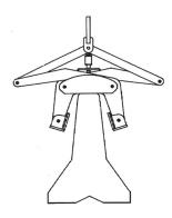
2. Raising crane hook will then cause pads to engage barrier.
