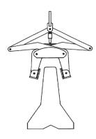
1. Grab in open position is placed onto barrier. Autolatch will disengage when hoist line becomes slack.
