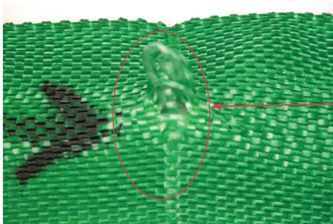
**THE DAMAGE:** Holes/Snags/Pulls exposing internal core yarns.
