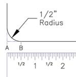
Minimum Edge Radii suitable for contact with unprotected polyester roundslings.
