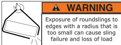
Edges do not need to be “sharp” to cause failure of the sling. The following table shows the minimum allowable edge radii suitable for contact with unprotected roundslings. Chamfering or cutting off edges is not an acceptable substitute for fully rounding the edges to the minimum radius. Slings can also be damaged from contact with edges or burrs at the sling connection.
