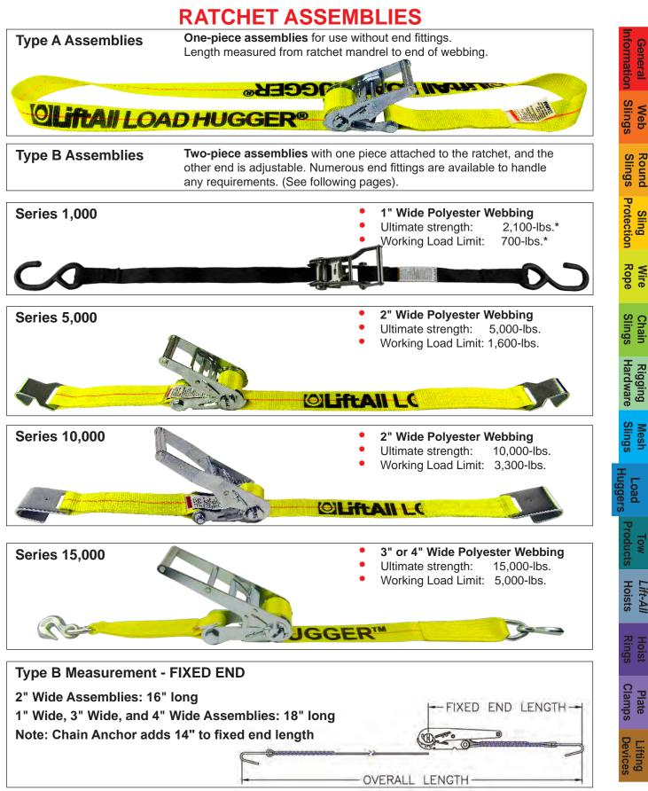
\* Series 1,000 Exception: Series 1,000 Ratchet Assembly with Flat Hooks, Ultimate Breaking Strength is 1,000-lbs. and Working Load Limit is 330-lbs.
