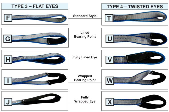
Textured, wear-resistant material is standard for these eye treatments. Other pad materials are available in the Sling Protection section of this catalog.
