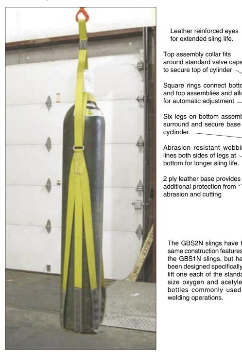
Leather reinforced eyes GBS1N for extended sling life. Top assembly collar fits around standard valve caps to secure top of cylinder Square rings connect bottom and top assemblies and allow for automatic adjustment -Six legs on bottom assembly surround and secure base of cvclinder. \_\_\_\_ Abrasion resistant webbing lines both sides of legs at bottom for longer sling life.
