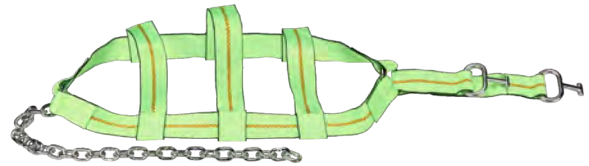
Cage Strap 2" Web • T-Hooks, 1/4"X26" G30 Chain WLL 1,600-lbs. **Used on Chevron ® and Challenger ® wheel lifts**
